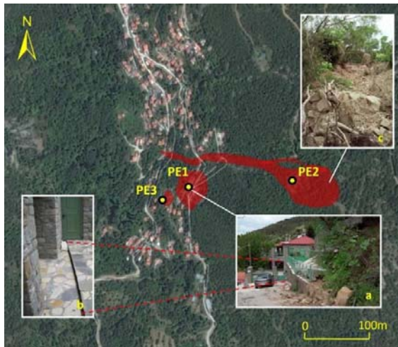
Figure 3: General View of the Perista village and the identified landslides : a) rotational landslide affecting a residence (PE1), b) Detail of the differential movement that was observed in the house in PE1 position, c) Complex landslide which took place outside of the village (PE2).
